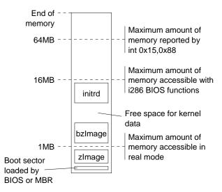
Figure 7: Simplified memory layout at boot time on i386.
