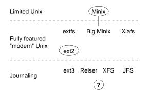
Figure 6: Evolution of the "standard" Linux file system.
