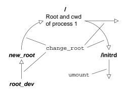
Figure 11: Changing the root file system with change\_root.
