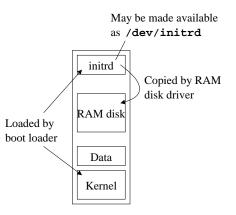
Figure 10: Loading an initial RAM disk.
