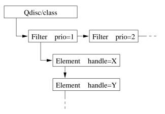
Figure 7: Structure of filters, with a list of elements belonging to the first filter, and no internal structure for the second filter.
