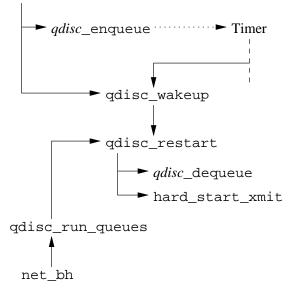
Figure 6: Functions called when enqueuing and sending packets.
