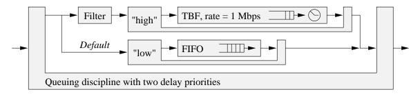
Figure 4: Combination of priority, TBF, and FIFO queuing disciplines.
