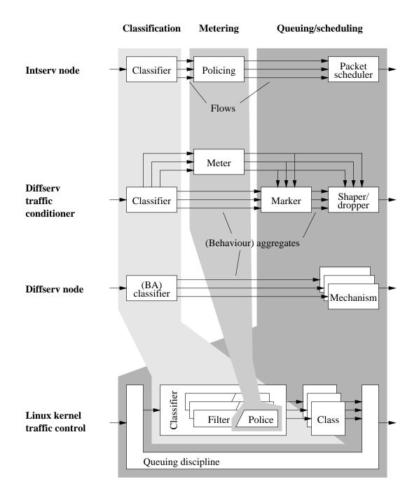
Figure 5: Relation of elements of the intserv and diffserv architecture to traffic control in the Linux kernel.
